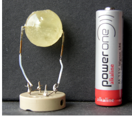
Figure 4.6 A photo of one of the spheres used in the measurements. At the time of the photo shoot (1 month after molding) the sample is no longer transparent - it has crystallized.
