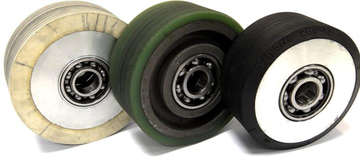
FIG. 3. Picture of the four test wheels. From the left: Nitrile butadiene rubber (NBR); Polyurethane (PUR); Continental truck tyre rubber mixture (CON).
