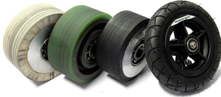
**Figure 5.12:** Picture of the used test wheels. From the left; Nitrile butadiene rubber (NBR), Polyurethane rubber (PUR), Continental Rubber (CON) and Powerslide CST 150 Air Tire (POW).
