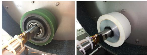
Fig. 3. Photos of the two test wheels used in this study. (a) Commercial polyurethane rubber (PUR) pallet truck wheel. (b) Custom made nitrile butadiene rubber (NBR) wheel.
